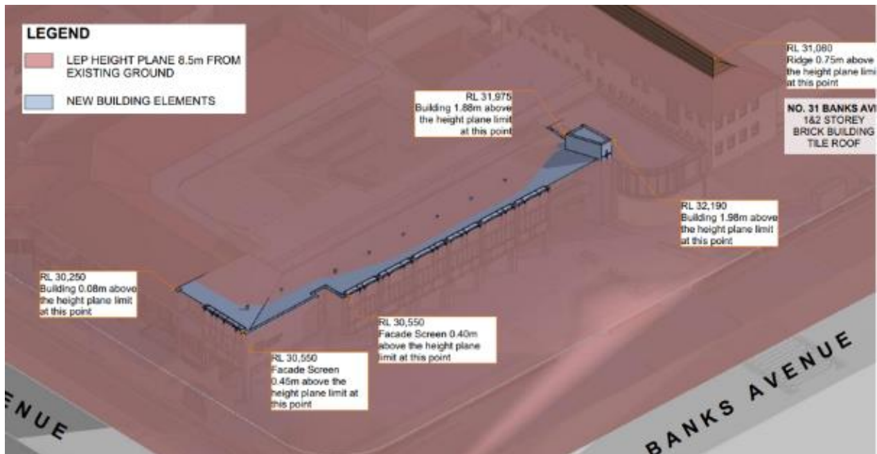
Figure 2: Portions of the protruding above the 8.5m building height plane (shown in red) are identified in blue above.
